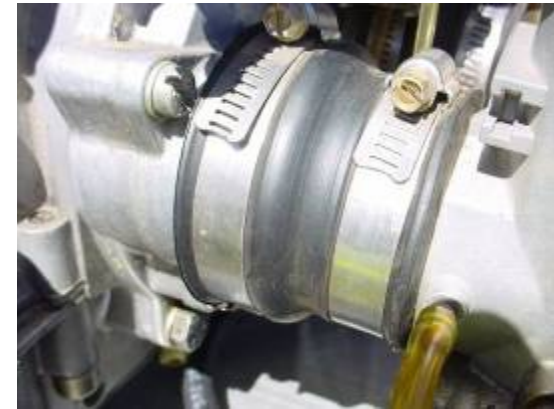
Over tight Wrong clamps
