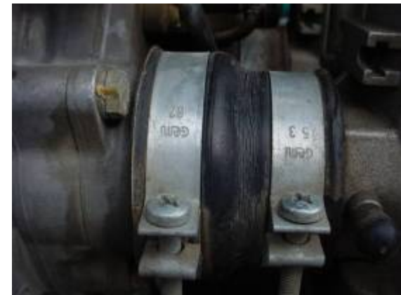
Intake socket cracks 2 stroke
