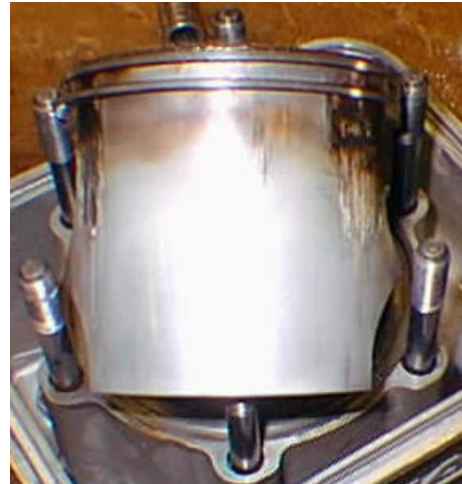
Cold seizure on exhaust side (PTO) of the piston.
