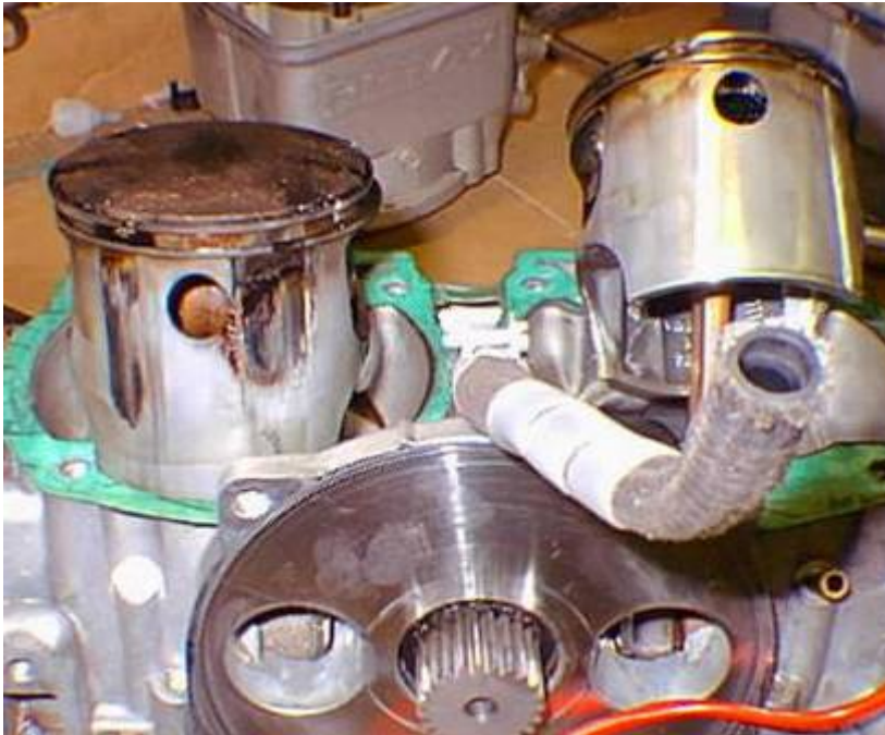
Cold seizure on Rotax 582 intake side of the piston.
